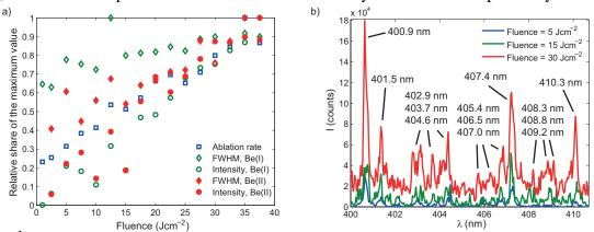
Figure 1: a) The behavior of the intensities and widths of Be(I) and Be(II) lines and the ablation rate of the studied coating as a function of the laser fluence, b) W(I) lines measured with different fluences, showing the increasing quasi background due to the weak W(I) lines around the most intense lines at 400.9 nm, 407.4 nm, and 410.3 nm.
