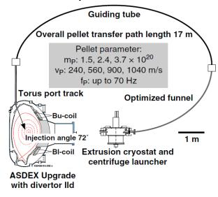
reported here where performed in the campaign 2012/13 concluding operation in the divertor IId configuration. The high speed inboard launching system, based on a centrifuge accelerator and a looping transfer system, was recommissioned
