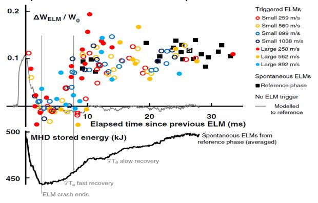
Figure 3: Upper: Relative loss of plasma energy versus time elapsed since onset of the previous ELM. Data obtained for different pellets and from spontaneous ELMs. The modelled response a pellet causing no impact on the ELM cycle is displayed a solid grey line. Lower: Averaged plasma energy evolution during a spontaneous ELM cycle.
