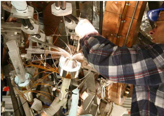
Fig. 3. The Joint Assembly - Connection of Strands
