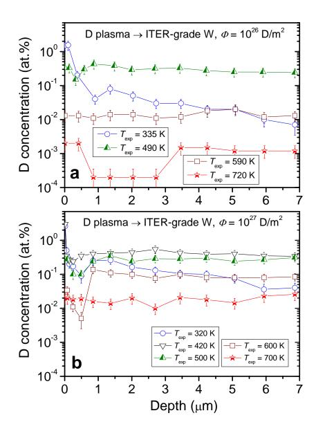
Figure 4. Depth profiles of deuterium retained in polycrystalline ITER-grade W exposed to low-energy (38 eV/D), high-flux ( $10^{22}$  D/m<sup>2</sup> s) D plasma with ion fluences of  $10^{26}$  (a) and  $10^{27}$  D/m<sup>2</sup> (b) at various temperatures.
