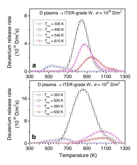
Figure 3. Thermal desorption spectra of deuterium released from polycrystalline ITER-grade W exposed to low-energy (38 eV/D), high-flux ( $10^{22}$  D/m<sup>2</sup> s) D plasma with ion fluences of  $10^{26}$  (a) and  $10^{27}$  D/m<sup>2</sup> (b) at various temperatures. The TDS heating rate was 0.5 K/s. Note that the deuterium release rate scales in panels (a) and (b) differ by a factor of 2.5.
