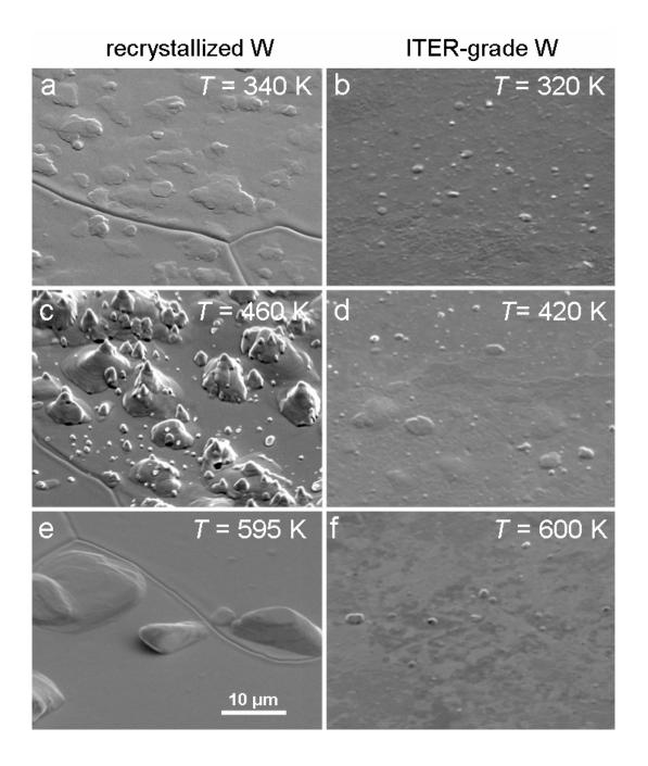
Figure 6. SEM images of recrystallized W (rc-W) (a, c, e – left part of the figure) [9, 15] and polycrystalline ITER-grade W (ITER-W) (b, d, f – right part of the figure) exposed to low-energy (38 eV/D), high-flux ( $10^{22}$  D/m<sup>2</sup> s) D plasma with an ion fluence of  $10^{27}$  D/m<sup>2</sup> at indicated temperatures. The scale bar given in panel (e) is valid for all images. The surfaces were tilted at an angle of 45° to the electron beam.
