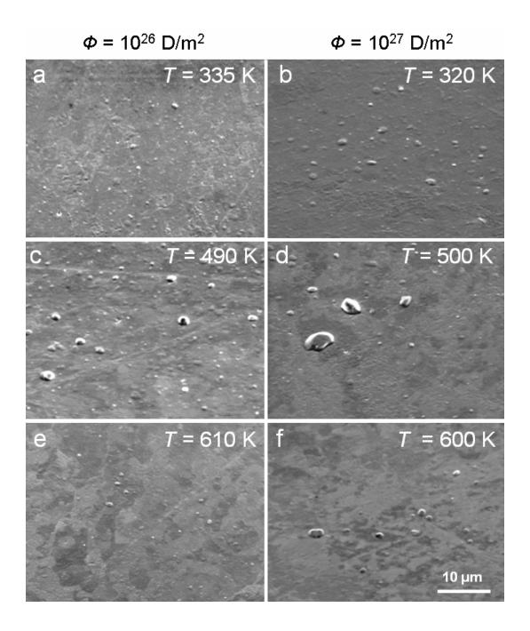
Figure 2. SEM images of polycrystalline ITER-grade W exposed to low-energy (38 eV/D), high-flux ( $10^{22}$  D/m<sup>2</sup> s) D plasma with ion fluences,  $\Phi$ , of  $10^{26}$  D/m<sup>2</sup> (a, c, e – left part of the figure) and  $10^{27}$  D/m<sup>2</sup> (b, d, f – right part of the figure) at indicated temperatures. The scale bar given in panel (f) is valid for all images. The surfaces were tilted at an angle of 45° to the electron beam.
