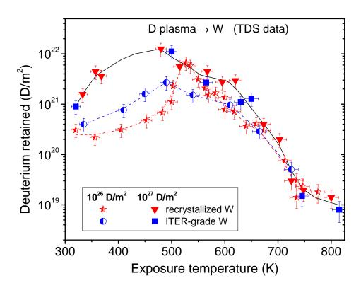
Figure 7. Total deuterium retention in recrystallized W [9, 15] and polycrystalline ITER-grade W exposed to low-energy (38 eV/D), high flux ( $10^{22}$  D/m<sup>2</sup> s) D plasma with ion fluences of  $10^{26}$  and  $10^{27}$  D/m<sup>2</sup>, as a function of the exposure temperature. The total deuterium retention was determined by thermal desorption spectrometry.
