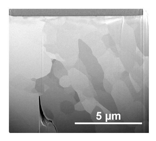
Figure 1. SEM/FIB cross section image of polycrystalline ITER-grade W (tilted by 38°).
