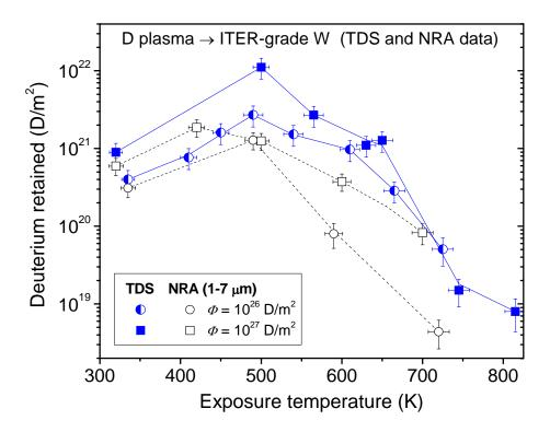
Figure 5. Deuterium retention in polycrystalline ITER-grade W exposed to low-energy (38 eV/D), high-flux ( $10^{22}$  D/m<sup>2</sup> s) D plasma with ion fluences of  $10^{26}$  and  $10^{27}$  D/m<sup>2</sup>, as a function of the exposure temperature. The total deuterium retention was determined by thermal desorption spectrometry (TDS) (filled symbols), whereas the D retention up to a depth of 7  $\mu$ m was measured by nuclear reaction analysis (NRA) (open symbols).
