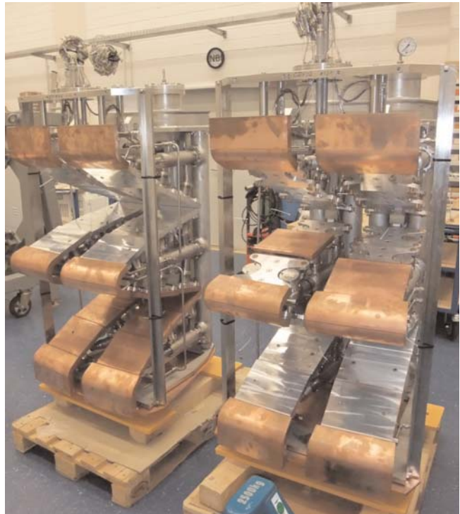
Figure 30: Calorimeter units, left: completed with target plates for the lower two beams and dummies for the upper two beams, right: target plates for upper two beams partially missing, dummies for the lower two beams installed.
