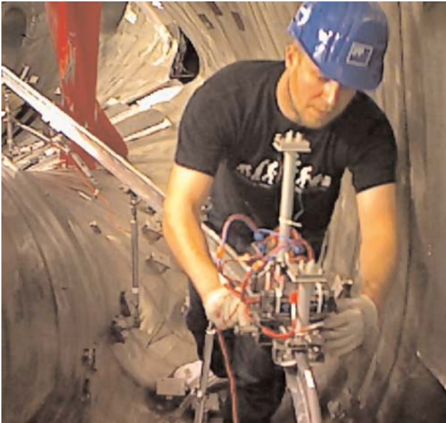
Figure 33: Neutron calibration test set-up in one W7-X module.
