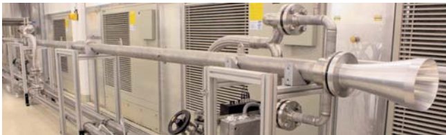
Figure 24: The “Long Load” in the ECRH-beam duct. The input taper is seen on the right.
