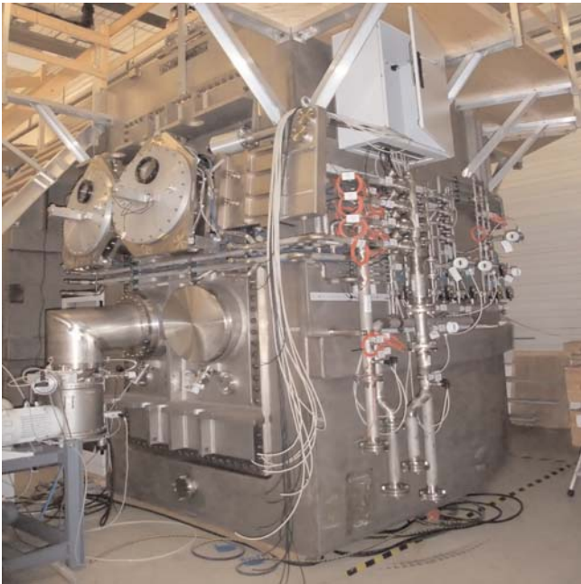
Figure 29: NBI 21 pre-assembled with source valves and beam steering units on the upper two source positions, a temporary vacuum system on one of the lower source ports, cooling manifolds, and instrumentation along the side.
