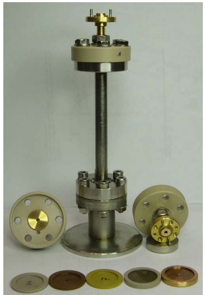
Figure 25: Vacuum interface prototype for the microwave waveguides with different types of sealing material.
