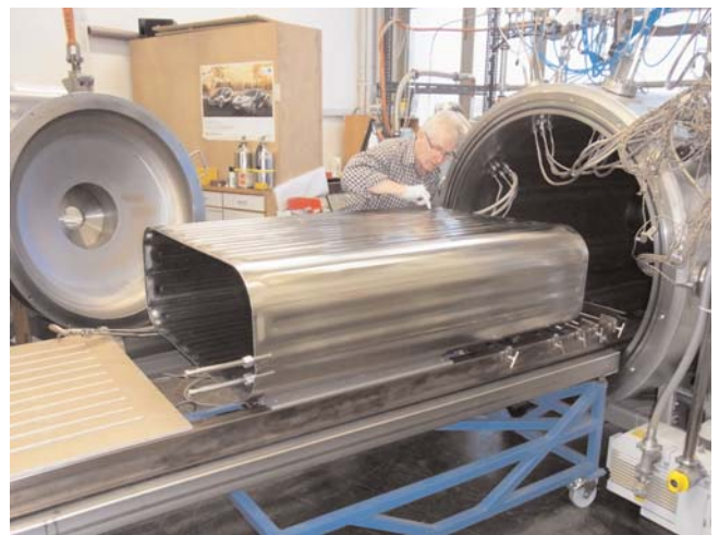
Figure 10: AEA v3 port protection panel prototype during testing at IPP Garching.
