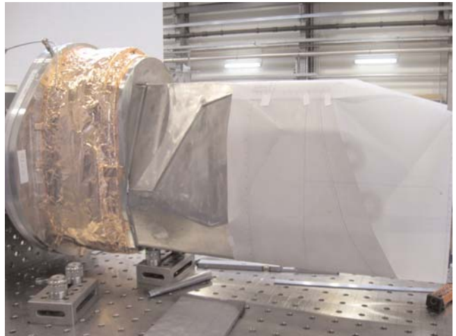
Figure 13: A NBI port prior to the contour cutting.
