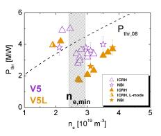
**Figure 5.** Variation of  $P_{th}r$  vs  $n_e$  with Be/W wall (2.4T/2.0MA) at low  $\delta$  for two divertor configurations with different strike point positions.
