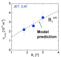
Figure 7.  $n_{e,min}$  variation vs  $B_T$  in JET with ILW.
