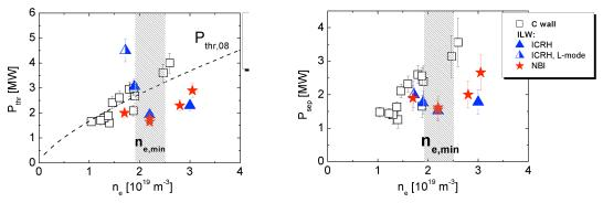
Figure 1. From left to right: Pthr and Psep at 1.8T/1.7MA for C and Be/W wall datasets.
