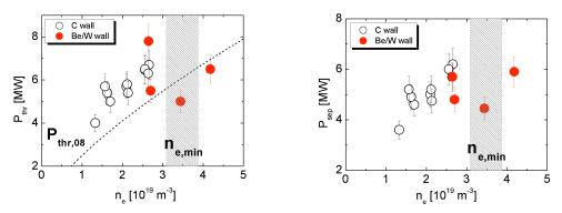
Figure 2. From left to right:  $P_{thr}$  and  $P_{sep}$  at 3.0T/2.75MA for C and Be/W wall datasets.
