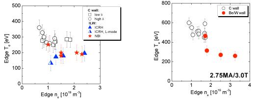
Figure 3. Edge Te vs edge ne at the L-H transition for C and Be/W wall: at 1.8T (left) and 3.0T (right).
