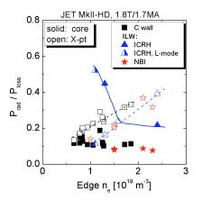
**Figure 4.** Radiated power, normalized to  $P_{loss}$ , at the L-H transition for C and Be/W wall (1.8T/1.7MA).
