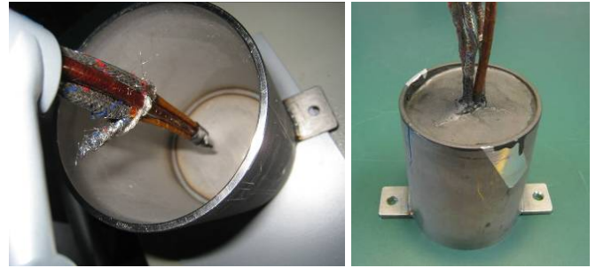
Fig. 3: Left side: Measuring cables and casting mold of the connecting piece before cast in. Right side: Not Paschen tight connecting piece after cast in, painted with conductive paint.
