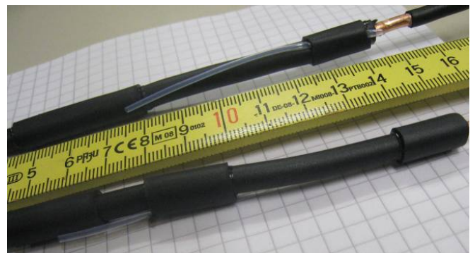
Fig. 4: Bare copper wire (right side), inner layer of heat shrinking tube and PVC-Tube, still without the outer layer of heat shrinking tube
