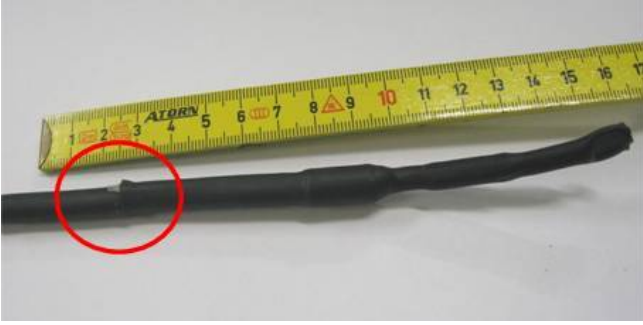
Fig. 5: Test object with outer layer of heat shrinking tube, outer end of the PVC-tube is free (on the left side)
