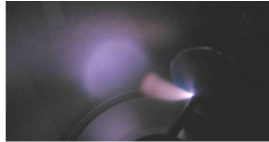
Fig. 12: The electric arc at 60 Pa
