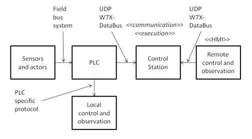
Fig. 2 Schema of PLC integration at W7-X
