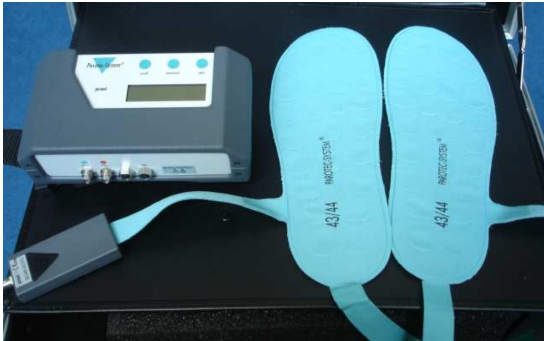
Figure 3.8.: Parotec insole pressure measurement system.
