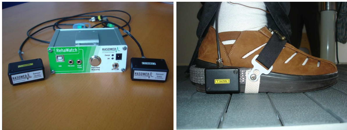
Figure 3.3.: Inertial sensor system: On the left the RehaWatch inertial sensor system is shown. On the right a brace and an ISU mounted on a foot are shown.
