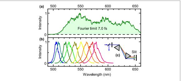
**Figure 1.** Performance of our NOPA system driven by picosecond pulses from an Yb:YAG disk laser. (a) Broadband output spectrum. (b) Tunable spectra with Fourier limits of ~40 fs for tunable photoemission studies. (c) Slit arrangement for spectral filtering in the Fourier domain.
