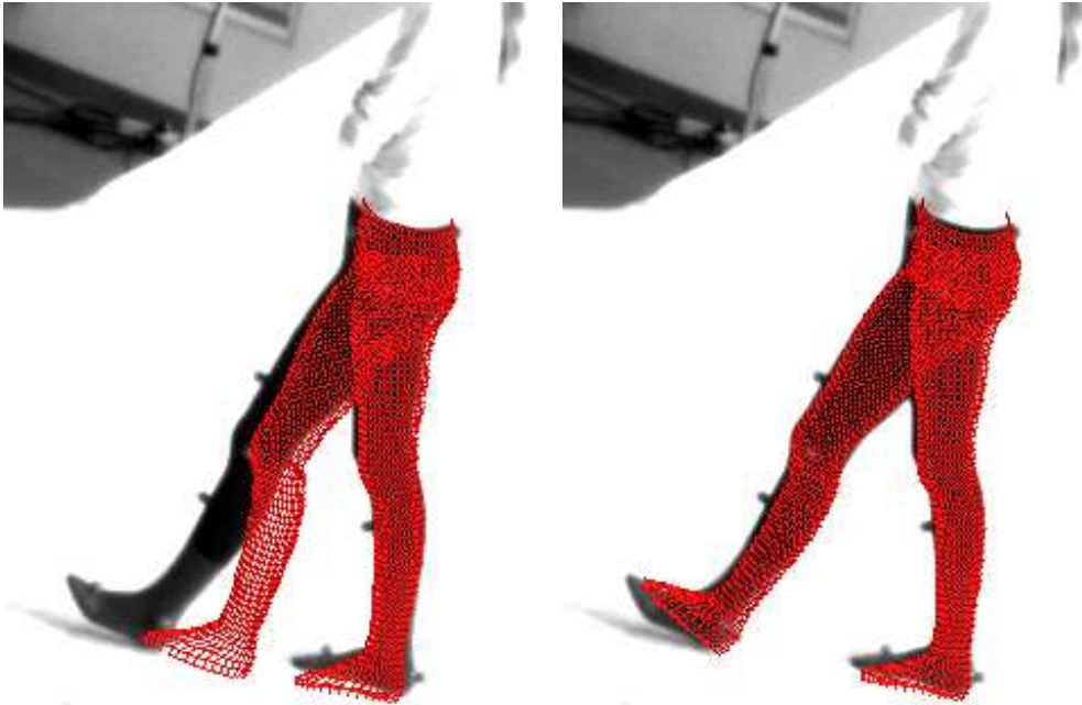
Figure 1.2: Motion capturing. Left: Estimate by a GPF with 2750 particles. Right: Estimate by an APF with 250 particles. The APF outperforms the GPF .
