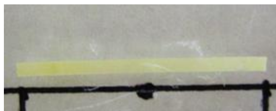
Figure S12. An optical photograph of a piece of PCMVImTf 2 N-PAA membrane (dense structure, without electrostatic complexation) placed in 1.5 mol% acetone-water mixture at 20 °C. Note: the membrane in Figure S12 was not painted with red color and shows its original yellowish color.
