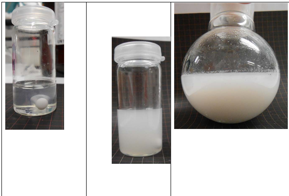
Photographs (from left to right): of the MF oligomer diluted in EtOH; basic reaction mixture upon addition of aqueous LUDOX HS-40 and the final dispersion.
