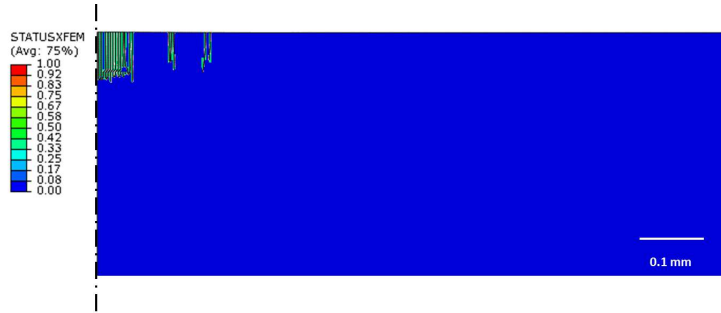
Fig. 24. Cracks predicted by XFEM simulation for a thermal shock load of 0.5 \text{ GW/m}^2 .
