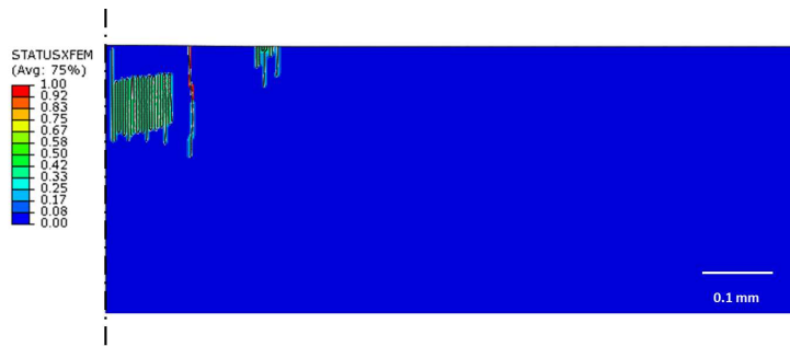
Fig. 25. Cracks predicted by XFEM simulation for a thermal shock load of 0.624 \text{ GW/m}^2 .
