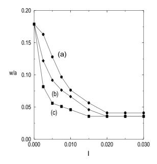
Fig.2 The saturated island width versus  $I=I_E/I_P$ , the relative amplitude of the driven current. Curve (a) is obtained with  $\Delta\eta$ =0, curve (b) with  $\Delta\eta$ =0.05, and curve (c) with  $\Delta\eta$ =0.1.
