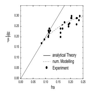
Fig.1  $\delta\beta/\beta$  versus the fraction of the bootstrap current density at the rational surface. For larger fra,  $\delta\beta/\beta$  saturates at 30% caused by a saturation of the island width for large fra.
