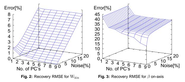
Fig. 2 shows the error for  $W_{kin}$ , the energy content of the plasma. Global quantities such as this, which depend on the volume-integrated magnetic field, are generally well recovered in the database. Indeed, the error is relatively low even for few added PC's, which is consistent with the fact that  $W_{kin}$  has an almost linear dependence on the plasma diamagnetic signal.
