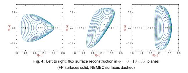
its simulated magnetic data. Fig. 4 compares the FP flux surface geometry to that of NEMEC for 3 different values of the toroidal angle  $\phi$ . The RMS deviation of the flux surfaces are representative of the average in the database, which decreases from 7mm at the centre to 3mm at the edge. The time taken for reconstruction of 11 flux surfaces (for s = 0.0, 0.1, ..., 1.0) is less than 20ms on a 143MHz UltraSPARC workstation.
