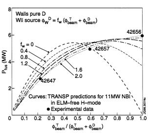
Fig. 2. Predicted and achieved  $\mathsf{P}_{DT}$  versus beam mix for an ELM-free plasma 11MW NBI, versus beam
