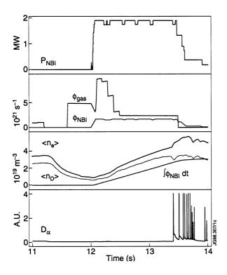
**Fig. 1.** Time traces for a high performance ELM-free discharge #40305 in deuterium; 3.8MA, 3.4T, 19MW NBI (+ 3MW ICRH, not shown) -mix and  $f_W$
