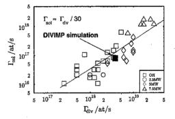
Figure 2 Correlation of the tungsten flux at the midplane scrape-off layer derived from deposition measurements to the tungsten erosion flux measured spectroscopically at the outer target plate.
