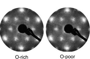
Figure 4: TDS spectra (m/e=32, O<sub>2</sub>) of 1 ML Figure 5: LEED patterns of O-rich and O-poor with biphase termination. The heating rate was energy used in the LEED experiments was 66 eV. 1.5 K/s. The upper panel displays the spectra on an expanded (5x) ordinate scale; the zero intensity line is shown below the curves.
