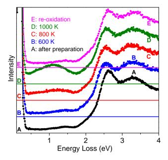
Figure 3: Electronic excitation spectra recorded in specular geometry of (A) an as-prepared  $Fe_2O_3$  film and spectra obtained after a subsequent short flash to 600 K (B), 800 K (C), 1000 K (D) and a final reoxidation step (E). The spectra are normalized such that the state at ~3.3 eV has the same intensity in all spectra. For clarity the curves are plotted with a constant y offset between successive graphs; the zero lines are shown and labelled with the label of the respective spectrum.
