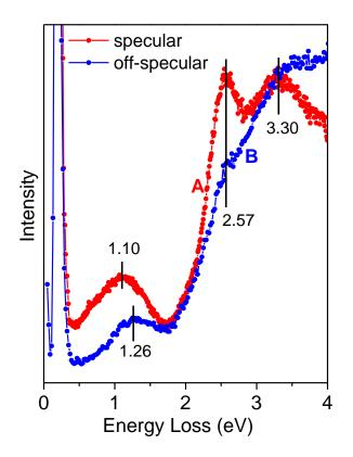
Figure 6: Electronic excitation spectra of *O-poor* biphase  $Fe_2O_3$  recorded in specular (curve A) and 10° off-specular (curve B) geometry. The two spectra were normalized such that the loss peak at 3.30 eV has equal intensity in both spectra.
