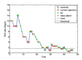
Fig. 2. An example of staircase from the study (condition "+Sway"). The initial roll rate was 12 deg/s, with initial step size 2 deg/s, which was halved to 1 deg/s after four reversals and to 0.5 deg/s after 8 reversals. The staircase was terminated after 12 reversals and the last five were averaged to compute the threshold (dashed line).
