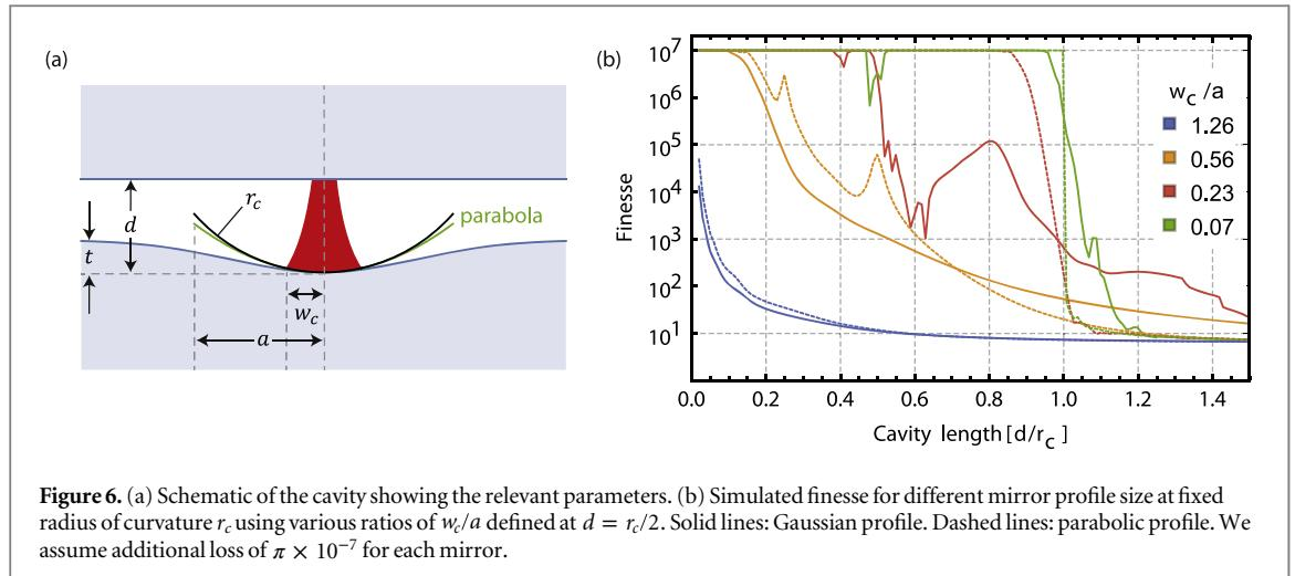
**Figure 6.** (a) Schematic of the cavity showing the relevant parameters. (b) Simulated finesse for different mirror profile size at fixed radius of curvature  $r_c$  using various ratios of  $w_c/a$  defined at  $d = r_c/2$ . Solid lines: Gaussian profile. Dashed lines: parabolic profile. We assume additional loss of  $\pi \times 10^{-7}$  for each mirror.
