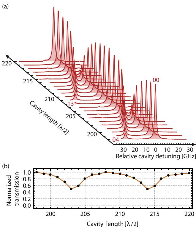
**Figure 4.** (a) Measured cavity transmission spectra as a function of relative cavity detuning. Wavelength: 856 nm. Avoided crossings between the fundamental mode and the fourth order modes 04 and 13 are visible. (b) Maximal transmission of each of the spectra shown in (a), normalized to the largest value.
