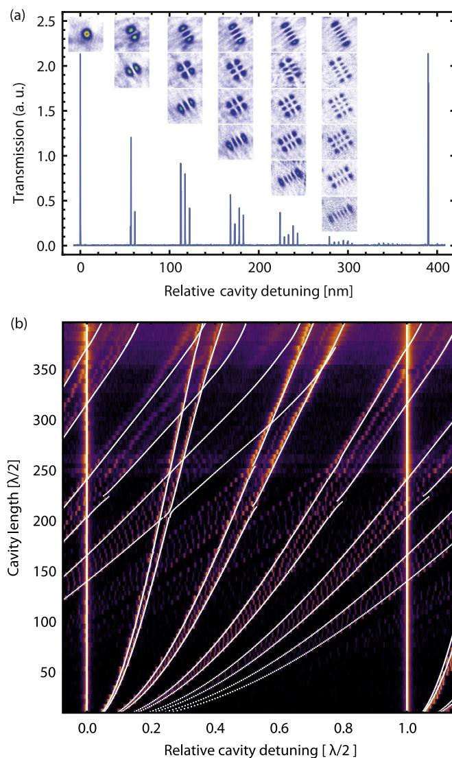
**Figure 3.** (a) Cavity transmission spectrum as a function of relative cavity detuning covering one free spectral range, where  $F \approx 60.000$ . The insets show the mode functions as measured by scanning cavity microscopy. Wavelength: 780 nm. (b) Cavity transmission spectra as a function of axial mode order  $q$  for  $F \approx 1200$ . Logarithmic color scale. Wavelength: 856 nm. White: model for modes  $(0, m + n)$  and  $(m + n, 0)$ .
