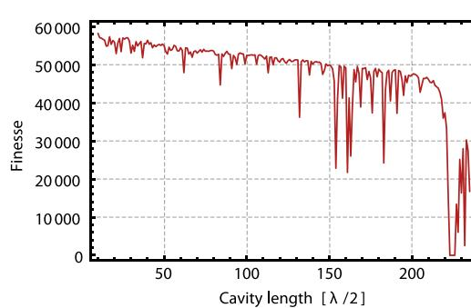
**Figure 2.** Cavity finesse as a function of axial mode order determined from measurements at 25 different positions within an area of  $30 \times 30 \mu\text{m}$  on a large planar mirror and taking the most prevalent values. Wavelength: 780 nm.
