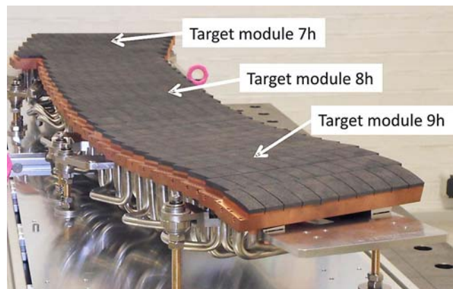
Figure 3: The plasma facing surface of the three high iota tail modules.
