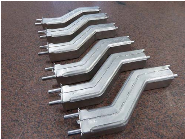
Figure 5: Cryopump parts after high temperature heat treatment.
