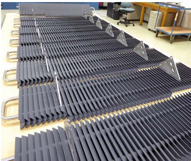
Figure 6: Water baffles after coating with an ECRH absorbent layer.
