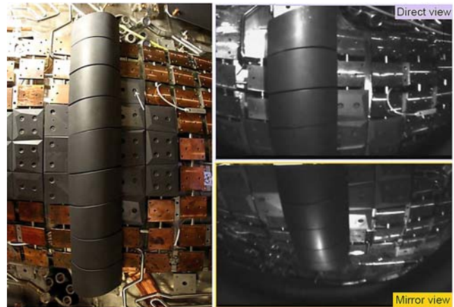
Figure 20: Video observation of the ECRH heat shield and the in-board limiter. Left: Picture of ECRH-heat shield and the in-board limiter inside the plasma vessel. Right: View of the NIR-video camera in the immersion tube with the direct view at the top and the mirror view at the bottom.
