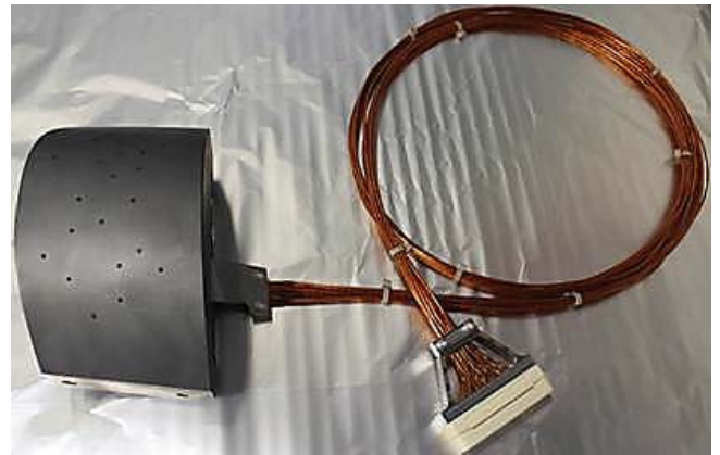
Figure 37: One of the limiter tiles with embedded Langmuir probes, before it was installed on Wendelstein 7-X.
