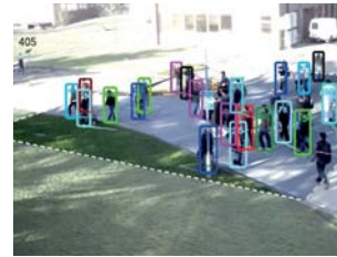
Figure 3 and 4: Example results obtained with our method for joint detection and tracking of people in crowded scenes
