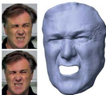
Figure 2: From video frames of only 2 cameras (left) we can reconstruct a detailed dynamic 3D model of the face (right).
