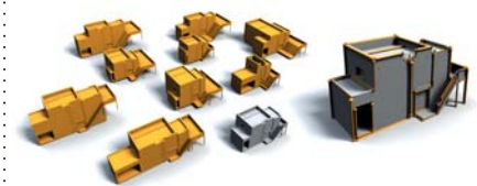
Figure 4: Building blocks (as in Figure 1) can be reassembled automatically to create plausible shape variations from a single example.
