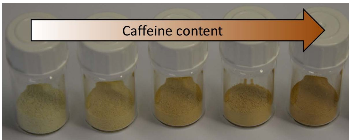
Figure S5. Images of the CM carbon nitride-materials with 0 mol-%, 2.5 mol-%, 5 mol-%, 7.5 mol-% and 10 mol-% caffeine added to the precursor mixtures (from left to right).
