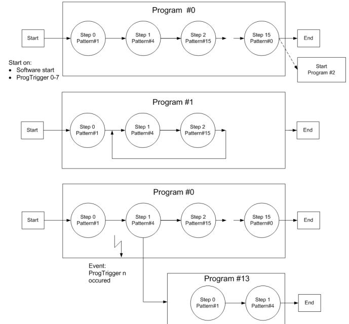
Fig. 4: Program examples for pulse sequences of a PSG
