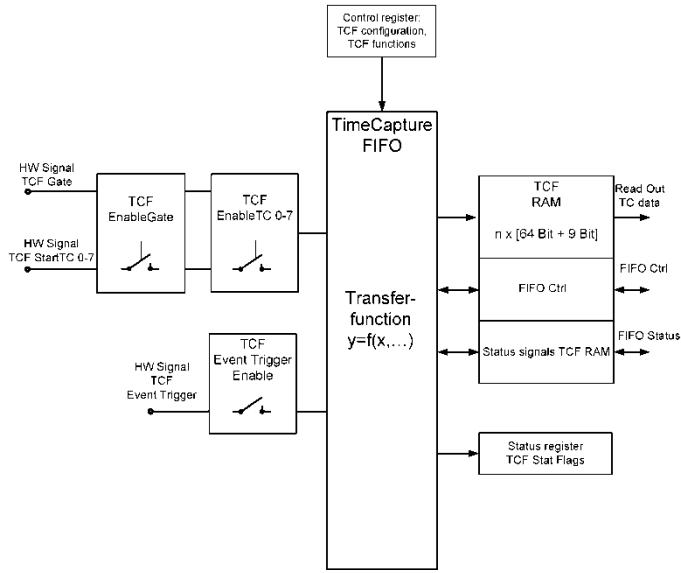
Fig. 2: Structure of the TCF device
