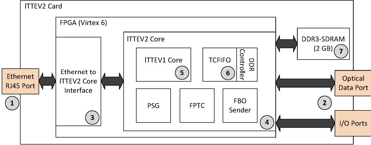
Fig. 1: System architecture of the ITTEV2 card
