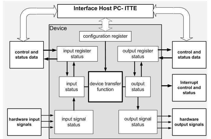
Fig. 2: System Generic model of a TTE device
