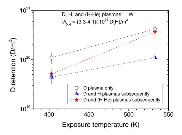
Figure 3. Amount of deuterium retained at depths of up to 8  $\mu$ m in recrystallized W exposed at the same temperature to D plasma only, to D and H plasmas sequentially, and to D and (H-He) plasma sequentially with fluences of  $3.3\times10^{24}$  D(H)/m<sup>2</sup> ( $T_{\rm exp}=403$  K) and  $4.1\times10^{24}$  D(H)/m<sup>2</sup> ( $T_{\rm exp}=533$  K), as a function of the exposure temperature.
