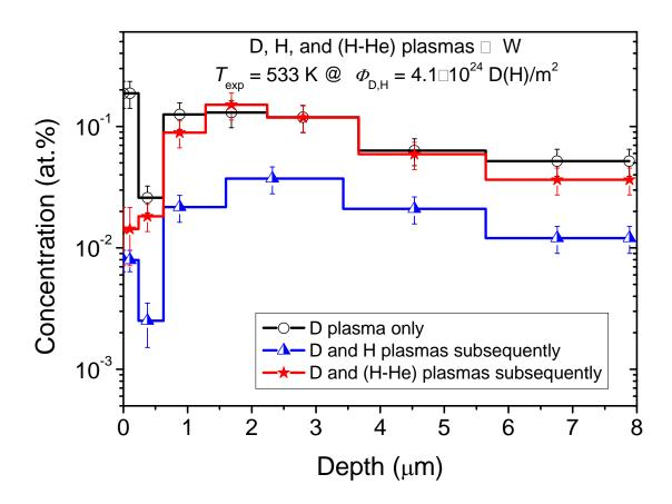
Figure 2. Depth profiles of deuterium retained in recrystallized W exposed at 553 K to D plasma only, to D and H plasmas sequentially, and to D and (H-He) plasma sequentially with the same fluence of  $4.1 \times 10^{24}$  D(H)/m<sup>2</sup>.
