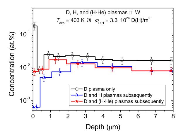
Figure 1. Depth profiles of deuterium retained in recrystallized W exposed at 403 K to D plasma only, to D and H plasmas sequentially, and to D and (H-He) plasma sequentially with the same fluence of  $3.3 \times 10^{24}$  D(H)/m<sup>2</sup>.
