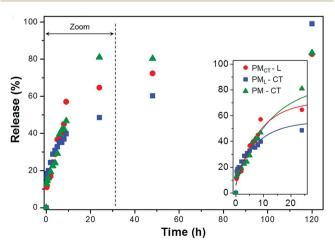
Fig. 6 R6G release percentage determined by fluorescent detection *versus* time for the different scaffolds (PM) in enzymatic media (L: lipase and CT:  $\alpha$ -chymotrypsin).
