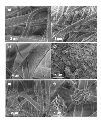
**Fig. 5** SEM micrographs of: (a) PCL scaffold after 412 h of immersion in DPBS medium, (b) PCL<sub>L</sub> enzyme loaded scaffold after 198 h of immersion in DPBS medium. (c) Sample PM-CT after immersion in  $\alpha$ chymotrypsin medium for 16 h and (d) 88 h. (e) Sample PM<sub>L</sub>-CT after immersion in  $\alpha$ -chymotrypsin medium for 48 h. (f) Sample PM<sub>CT</sub>-L after immersion in lipase medium for 48 h.
