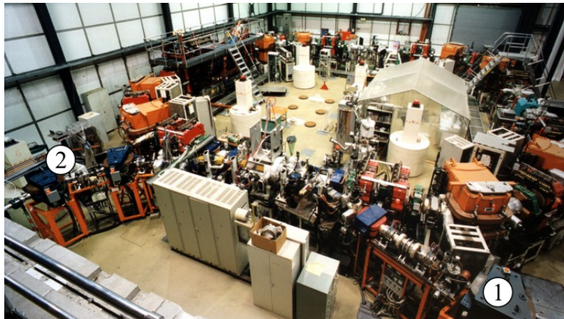
Figure 3.1.: Photography of the Heidelberg TSR, in operation until end of 2012. In the front section, the injection (1) and extraction (2) beam lines are shown.
