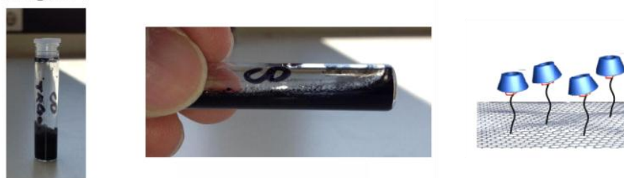
Figure S12. Photographs of a) ManCD@AG4 and b) CD@AG4 dispersed in Milli-Q water. With the functionalization of ManCD, the resulting ManCD@AG4 (98.2 \mu\text{M} , calculated based on \beta -CD unit) exhibits higher solubility in water. The ManCD@AG4 is homogenous black liquid. In the contrast, the CD@AG4 with identical concentration has limited solubility. Many agglomerates of fine particle are visible.
