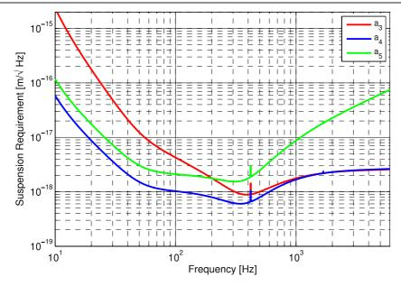
**Figure 5.** Suspension requirement for the maximum tolerable lateral grating displacement that is necessary to achieve the Advanced Virgo design sensitivity. The suspension required strongly depends on the actual readout port as well as the frequency of interest. At low frequencies the phase noise suppression in port  $a_3$  allows significant relaxation of the required suspension isolation. The narrow peak around 410 Hz is due to a resonance in the Advanced Virgo design, not a grating effect.
