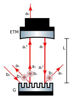
**Figure 3.** External input port  $b_0$ , internal input ports  $b_1$ ,  $b_2$ ,  $b_3$  (marked by encircled addition symbols) and transfer ports  $a_q$  in a grating cavity.
