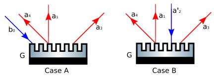
**Figure 2.** Input ( $b_0$ ,  $a'_2$ , shown blue) and output ( $a_1$ ,  $a_3$ ,  $a_4$ , shown red) light field amplitudes at a phase modulating grating in second order Littrow configuration in case A, and zeroth order Littrow configuration in case B (labels consistent with figure 3).
