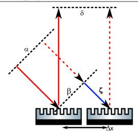
**Figure 1.** Wavefronts coupling through a diffraction grating. The wavefront (propagation vector shown in solid red) originates at  $\alpha$ , travels to  $\beta$  and is diffracted to  $\delta$ . When the grating is laterally displaced by  $\Delta x$ , the wavefront (propagation vector shown red dashed) must pass through additional path-length  $\zeta$  (propagation vector shown in solid blue).
