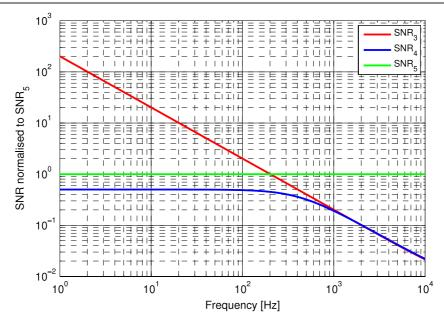
**Figure 4.** Signal to noise ratio of gravitational wave equivalent mirror displacement and lateral grating displacement at the three different output ports of a grating gravity. All traces are normalized to SNR<sub>5</sub>.
