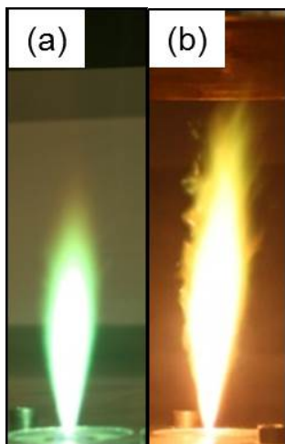
Figure 2. The flame pictures of 6\text{Cu}_3\text{Zn}_1\text{Al} -nitrate (a) and 6\text{Cu}_3\text{Zn}_1\text{Al} -organo (b).
