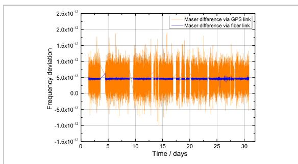
**Figure 5.** Frequency deviation between the two masers at MPQ and PTB measured over the GPS link and over the fiber link, respectively. The masers show a mean frequency difference of about  $4.6 \times 10^{-13}$  with respect to each other. The occasional gaps in the fiber link data are due to cycle-slips and a malfunction of one of the frequency comb systems. GPS link data are only shown at intervals when the fiber link data were available.
