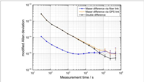
**Figure 4.** Frequency instability of the maser difference measured via the fiber link and via the GPS link, respectively. The double difference reveals the true GPS link performance without any contribution from the masers.
