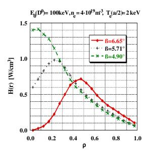
Fig. 2: NBI deposition profiles for three different injection geometries
