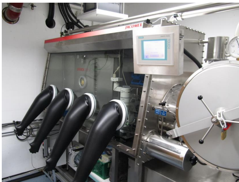
Figure 10.9. OFET measurement system inside glove box.
