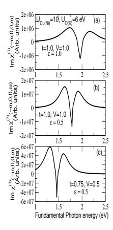
FIG. 5: Effect of lattice constant, charge transfer energy in isostructural one dimensional Mott-Hubbard insulators. For same values of on-site coulomb repulsions, in Fig (a)  $\epsilon = 1.0$ , V = t = 1 eV; in Fig (b)  $\epsilon = 0.5$  eV, V = t = 1 eV; and in Fig (c)  $\epsilon = 0.5eV = V$  t = 0.75 eV in order to simulate situation from  $Sr_2CuO_3$  to  $[Ni(chxn)_2Cl]Cl_2$  to  $[Ni(chxn)_2Br]Br_2$ .
