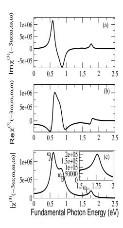
FIG. 1: Third order susceptibility of one-dimensional Mott-Hubbard insulators relevant to third harmonic generation. Imaginary part of the THG susceptibility (a), real part of the THG susceptibility (b), magnitude of the THG susceptibility (c). Locations of  $\omega_A$ ,  $\omega_B$ ,  $\omega_C$  are very close to the experimentally observed values. The peak at  $\omega_A$  is a three-photon resonant one whereas those at  $\omega_B$  and  $\omega_C$  are two-photon resonant.
