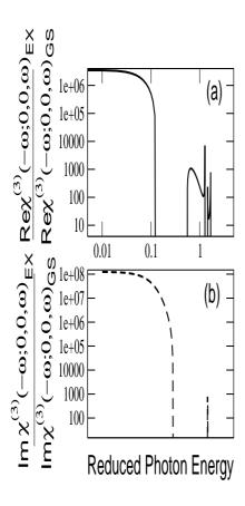
FIG. 8: Excited state enhancement of real (a) and imaginary (b) parts of the third order susceptibility with respect to the ground state relevant for EA in logarithimic scale.
