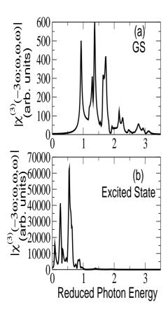
FIG. 9: Third harmonic generation (THG) susceptibility (a), excited state THG susceptibility (b) for poly-(paraphenylenevenylene) (PPV).
