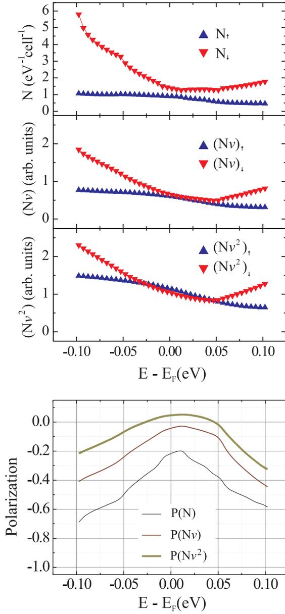
FIG. 6: (Color online) Spin dependent densities of states  $N$ , Sharvin conductance  $(Nv)$ , plasma frequencies  $(Nv^2)$  (upper panel), and the derived spin polarizations for the theoretical lattice constant of  $\text{CeMnNi}_4$  (lower panel).
