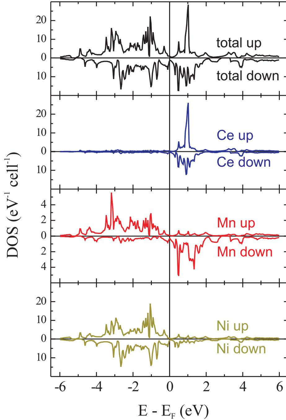
FIG. 4: (Color online) Total spin dependent DOS of CeMnNi<sub>4</sub> and the local DOS for Ce, Mn, and Ni (from top to bottom), respectively.
