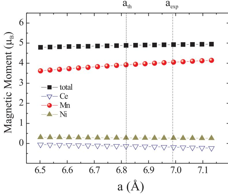
FIG. 2: (Color online) Total magnetic moment (black squares) as well as magnetic moments of Ce (open down-triangles), Mn (solid circles), and Ni (solid up-triangles) as a function of lattice constant of CeMnNi<sub>4</sub>. The vertical lines mark theoretical and experimental values of the lattice constant, respectively.
