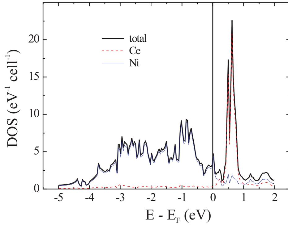
FIG. 3: (Color online) Total and partial density of states of the non-magnetic hexagonal CeNi<sub>5</sub>.
