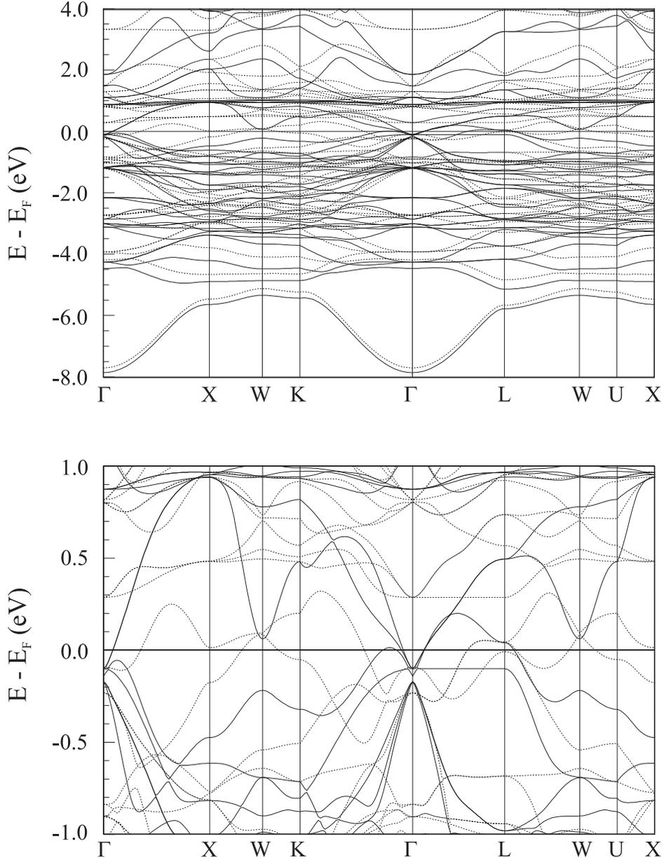
FIG. 5: The spin-resolved band structure of CeMnNi<sub>4</sub> over wide energy range (upper panel) and in the vicinity of Fermi level (lower panel). Solid and broken lines represent spin-up and spin-down electronic channels, respectively.
