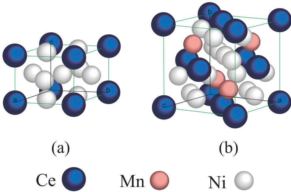
FIG. 1: (Color online) Crystallographic structures of (a) the hexagonal CeNi<sub>5</sub> and (b) the cubic CeMnNi<sub>4</sub> compound.
