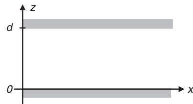
FIG. 5: Schematic drawing of the flow-cell seen from the side. The liquid is contained between the two glass cover-slips (shown in grey) at positions z = 0 and z = d .
