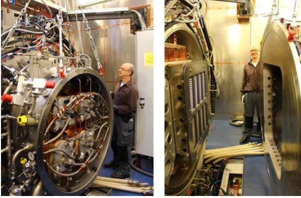
FIG. 1. (Color online). The RF driven ion source at the ELISE test facility. Left. View onto the RF drivers with dismantled vacuum dome. Right. Source opening with view onto the grid system and into the source chamber.
