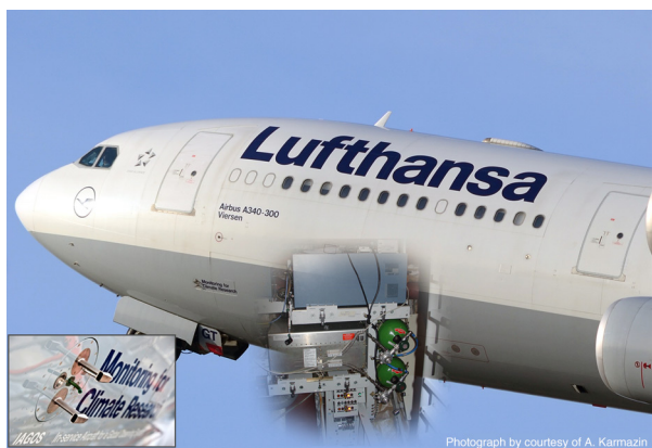
Fig. 2. IAGOS-CORE installation position aboard the Lufthansa A340-300 ‘Viersen’ (photograph by courtesy of A. Karmazin); the inset shows details of the IAGOS Inlet Plate, which carries the inlet probes for trace gas sampling (photograph by courtesy of Lufthansa).
