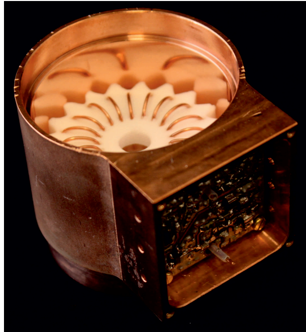
Figure B.3: Picture of the cyclotron coil inside the housing. The inner surface of the housing is mechanically polished.
