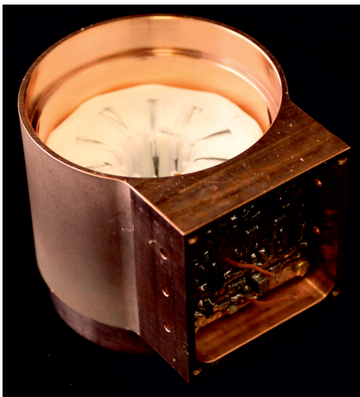
Figure B.1: Picture of the axial coil inside the housing. The two halves of the coil body are pressed together by wrapping several layers of PTFE tape around the outer spacers. The inner surface of the housing is mechanically polished.
