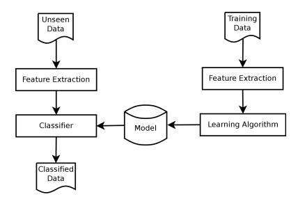
Figure 2.4: Data flow of a classification task in machine learning
