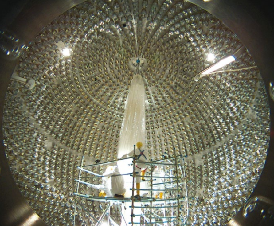
Fig. 11 Inside the BOREXINO with the photomultipliers arrays, while installing the inner balloon. Borexino Collaboration-LNGS/INFN.
