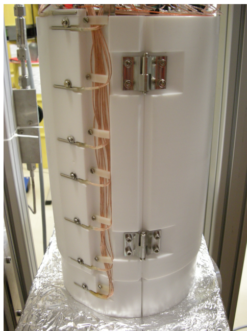
Figure 4.3.: (Left) View of the Pt100 sensors on the block's outside. (Right) Heights of the Pt100 sensors (relative to the block's bottom edge).
