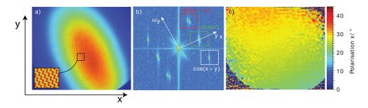
Figure 2: (a) interference pattern on the camera chip, (b) Fourier transform of the image and (c) MSE polarisation angle in 2D
