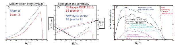
Figure 4: (a) Intensity of the beam signal at different radial locations, (b) resolution and pitch angle sensitivity versus plasma radius, (c) light cone reaching the IMSE backend
