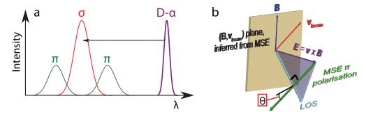
Figure 1: a:  $\pi$  and  $\sigma$  components of the MSE spectrum. b: 3D visualisation of the MSE principle: the  $\pi$  polarisation is the projection of **E** onto the plane perpendicular to the LOS. Knowing **E** lets us calculate the (**B**,  $\mathbf{v}_{beam}$ ) plane
