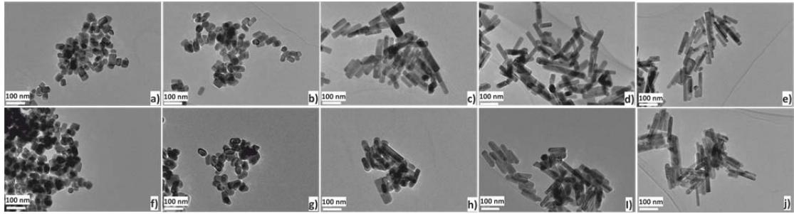
**Figure S4.** TEM micrographs of as-synthesized (top row) and at 400 °C thermally activated (bottom row) nanostructured MnWO<sub>4</sub> catalysts with different aspect ratio: 1.5 (a) and (e), 1.7 (b) and (g), 3.2 (c) and (h), 3.9 (d) and (i), 5.1 (e) and (j).
