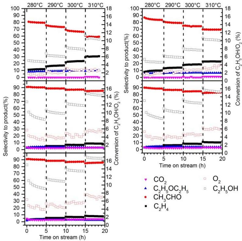
**Figure S7.** Catalytic performance of top-left) AR1.5, top-right) AR1.7, middle-left) AR3.2, middle-right) AR3.9, and bottom-left) AR5.1 sample in ethanol oxidation reaction at different temperatures; For reaction conditions see Experimental in the main text.
