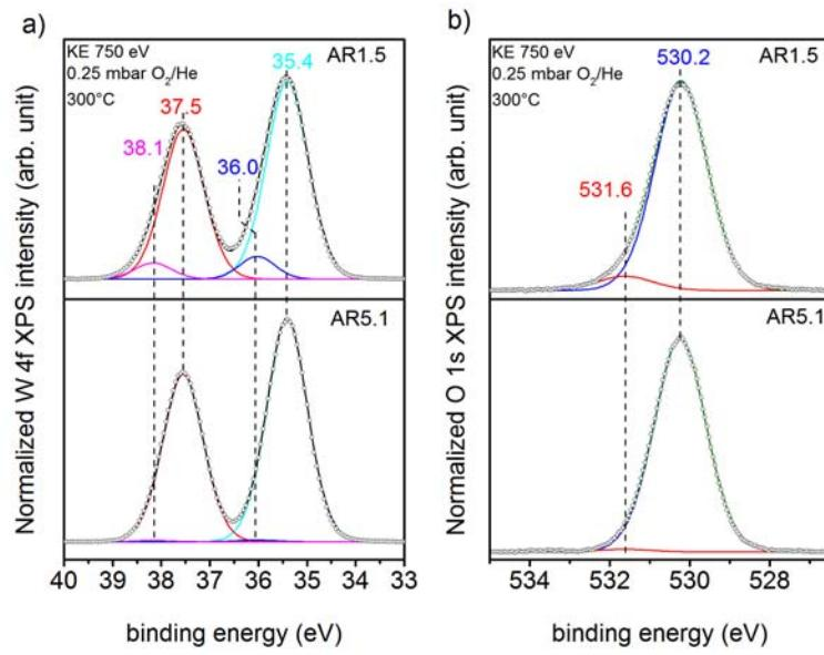
**Figure S10.** W 4f spectra (a)), and O 1s spectra (b)) of the catalysts AR1.5 and AR5.1 measured by synchrotron-based near ambient pressure X-ray photoemission spectroscopy (NAP-XPS) at an inelastic mean free path (IMFP) of ca. 1.6 nm in 0.25 mbar in O<sub>2</sub>/He at a total gas flow of 4.2 sccm at 300°C.
