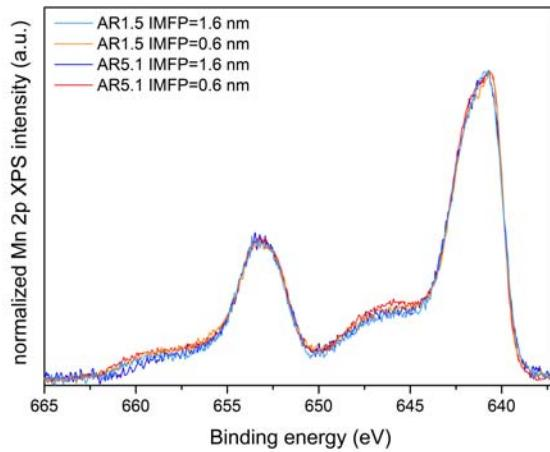
**Figure S11.** Mn 2p spectra of the catalysts AR1.5 and AR5.1 measured by synchrotron-based near ambient pressure X-ray photoemission spectroscopy (NAP-XPS) at an inelastic mean free path (IMFP) of ca. 0.6 nm (a) and 1.6 nm (b) in 0.25 mbar in O<sub>2</sub>/He at a total gas flow of 4.2 sccm at 300°C.
