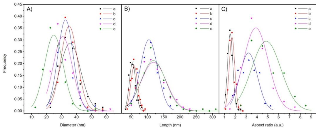
**Figure S5.** Distribution of A) diameter, B) length and C) aspect ratio of the nanostructured MnWO<sub>4</sub> catalysts after thermal treatment; In each plot, a, b, c, d, and e represent the catalysts AR1.5, AR1.7, AR3.2, AR3.9, and AR5.1, respectively.
