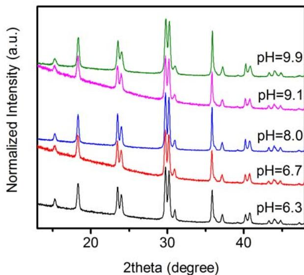
**Figure S2.** XRD patterns of the hydrothermal products; The pH of the starting solution is provided in the legend of the figure. For allocation of the corresponding final catalyst, please refer to Table 1 in the main text.
