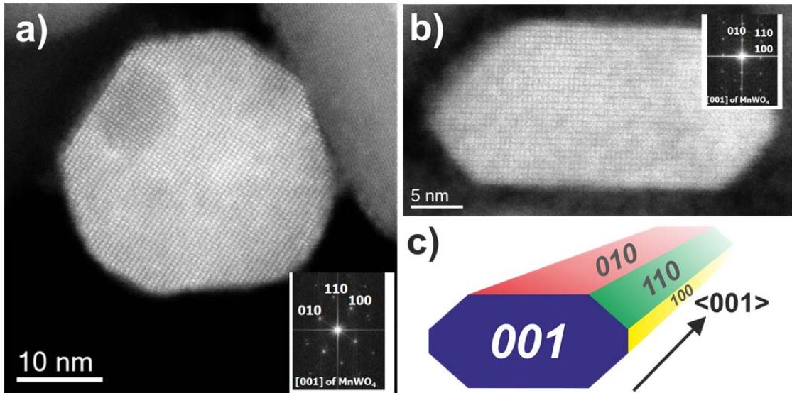
**Figure S6.** HAADF-STEM images of MnWO<sub>4</sub> nanoparticles viewed along <001> with different aspect ratios: a) AR1.5, b) AR5.1 and c) perspective model for a typical faceted nanoparticle.
