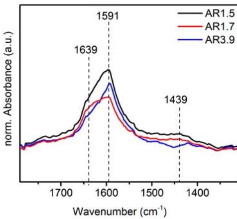
**Figure S9.** FTIR spectra of  $\text{NH}_3$  adsorbed at the surface of the catalysts AR1.5, AR1.7, and AR3.9 after pretreatment at 300°C for 1h in vacuum; Adsorption of ammonia was performed at 40°C; The spectra have been recorded in presence of gas phase ammonia ( $p=6.508\text{-}7.042 \text{ mbar}$ ).
