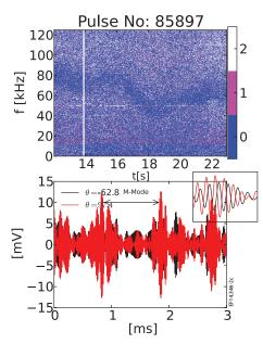
Figure 2: Top:Toroidal mode spectrum. Bottom: zoom on two  $\dot{b}$  probe, located at different poloidal position, pass-band filtered between 60 and 80 kHz. The inset magnify the two signals to highlight the poloidal periodicity
