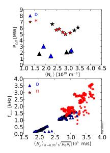
Figure 5: Top: L-H Power threshold vs density for Hydrogen and Deuterium discharges. Bottom: scaling of the M-Mode frequency vs Poloidal alfven speed. The color code is consistent with the top panel
