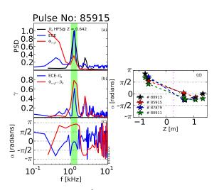
Figure 3: (a) PSD of  $B_{\theta}$  (black), ECE Channel (blue),  $\Phi_{refl}$  (red). Coherence (b) and Phase (c) between integrated magnetic and ECE (blue) and magnetic Reflectometer (red). (d) Phase between ECE and Magnetic field at different Z computed at the M-Mode frequency
