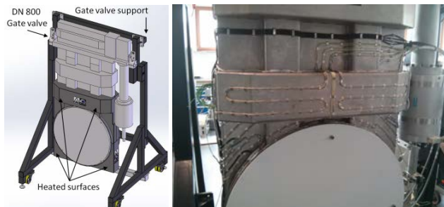
Figure 5: Left: CAD model of new DN 800 VAT gate on support structure with indication of heated surfaces. Right: detail of the new gate valve during testing of heating system, without thermal insulating jacket and with visible heating elements and cabling.
