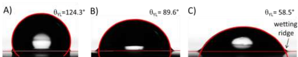
Figure 3. Drops deposited on a lubricant-infused textured surface. A) Water, B) ethylene glycol, and C) hexadecane drops were placed on inverse opals infiltrated with FC70. The circular red line represents a fit of the drop contour to the Young–Laplace equation. The angles were obtained by fitting the contour of the drop using a Young-Laplace fit. The volume of each drop was 3 \mu\text{L} .
