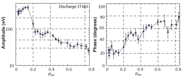
**FIGURE 3.** Radial profile of the amplitude and phase of the ion temperature modulation with respect to the applied ICRF power modulation as deduced from CXSR measurements in discharge 31563 at a plasma current of 0.6 MA and a magnetic field of 3 T.
