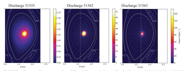
**FIGURE 6.** Tomographic reconstruction of 2D soft X-ray emission profiles for discharges 31555, 31562 and 31563 with NBI only, with NBI and off-axis <sup>3</sup>He minority heating, and with NBI and on-axis <sup>3</sup>He minority heating, respectively. Note the large differences in the maximum emissivities as indicated by the color bars.
