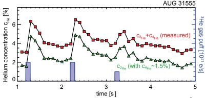
**FIGURE 1.** Time evolution of the measured total He concentration( $\square$ ) and the estimated <sup>3</sup>He concentration ( $\Delta$ ) with respect to  $n_e$  in discharge 31555. Also shown are the <sup>3</sup>He puffs applied at t = 1.2 s, 2.2 s and 3.2 s.
