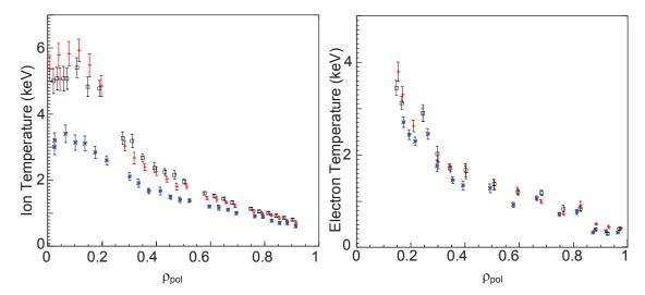
**FIGURE 8.** Radial  $T_i$  profile as measured by CXRS and radial  $T_e$  profile as measured with Thomson scattering as a function of  $\rho_{pol} \approx r/a$  at t = 3.1 s (+) and t = 3.4 s ( $\square$ ) for discharge 31585 and at t = 3.1 s for discharge 31587 (\*). The  $^3$ He concentration was 6 and >10% in discharge 31585 and 31587, respectively.
