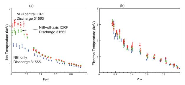
**FIGURE 4.** (a) Radial ion temperature profile as measured with CXSR and (b) radial electron temperature profile as measured with Thomson scattering at t=3 s for discharge 31555 with NBI only, discharge 31563 with NBI and central ICRF and discharge 31562 with NBI and off-axis ICRF as a function of  $\rho_{pol} \approx r/a$  where r/a is the normalized plasma minor radius. The symbols in (b) are the same as in (a).
