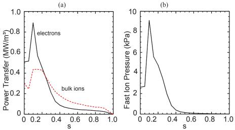
**FIGURE 7.** Radial profile of (a) ICRF power transferred to bulk ions and electrons and (b) pressure of the ICRF-accelerated fast  ${}^{3}$ He ions as given by PION for discharge 31563 at t = 3.1 s. Here, s  $\approx$  r/a is the square root of the normalized poloidal flux.
