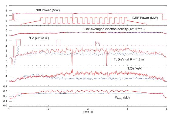
**FIGURE 2.** Overview of plasma parameters for discharges 31555 (dashed, blue online) with NBI only and for discharge 31563 (solid, red online) with NBI and ICRF heating tuned to a central  ${}^{3}$ He resonance at  $R_{res} \approx 1.65$  m (corresponding to  $x/a \approx -0.1$ ).
