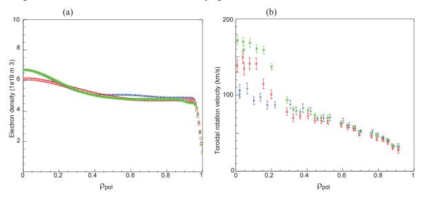
**FIGURE 5.** (a) Electron density profile and (b) plasma toroidal rotation profile as measured with CXSR at t = 3 s for discharge 31555 with NBI only, discharge 31563 with NBI and on-axis ICRF, and discharge 31562 with NBI and off-axis ICRF as a function of  $\rho_{pol} \approx r/a$ . The symbols are as in Figure 4.
