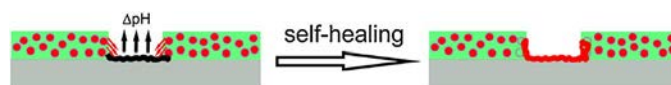
Fig. 7. Schematic presentation of the corrosion protection behaviour of the polyepoxy powder coatings with 8-hydroxyquinoline loaded nanocontainers.
